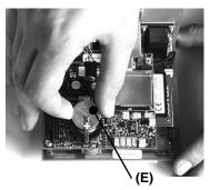
Fig. 2.5.6 Replace the battery (E). Observe right polarity.
