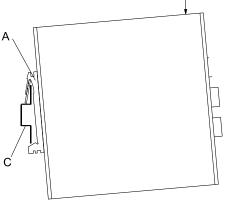
For dismounting, press in the direction of the marked point D while pulling at the bottom of the HECPM in direction E, Fig. 2.3.3.
