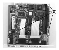
Fig. 2.5.4 Remove the 4 screws (D).
