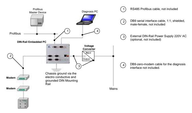
Fig. 2.4: Electrical Installation - Circuit Diagram
