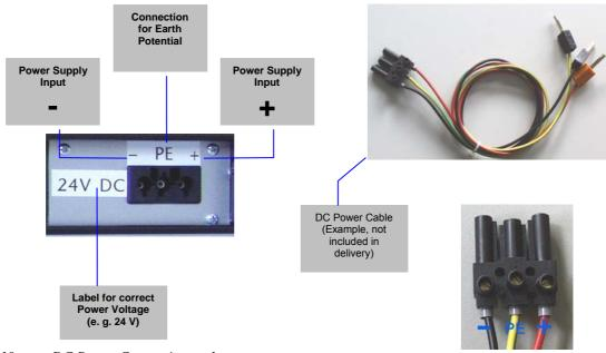
Figure 10. DC Power Connection socket
