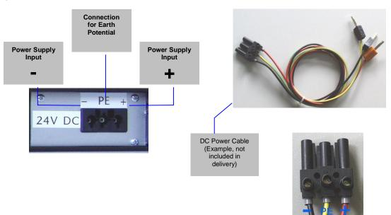
Figure 10: DC Power Connection socket
