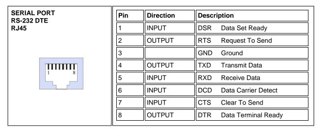
Figure 5: Pin Assignment of RJ45 interface (Communication Board)
