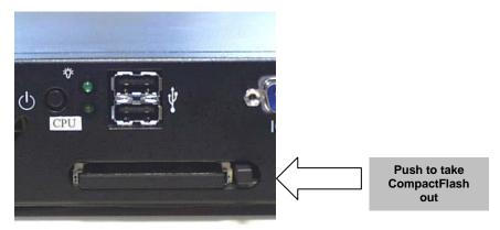
Figure 7: CompactFlash Adapter
