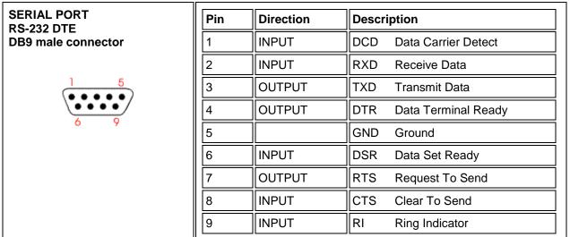
Figure 3: Pin Assignment of DB9 Interface (Computer) COM1-COM2
