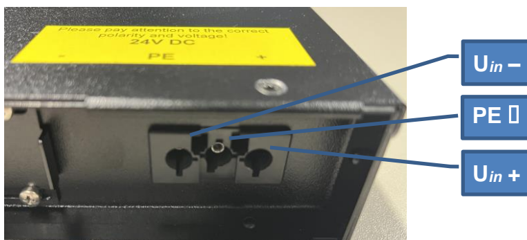
Figure 12: DC voltage connection at the power supply
