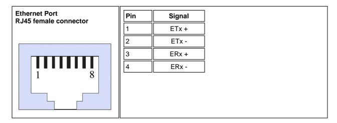
Figure 7: Pin assignment of Ethernet RJ45 interface
