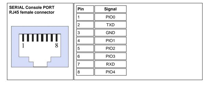
Figure 8: Pin assignment of RJ45 interface of serial console port
