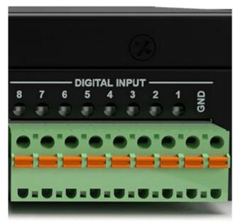
Figure 15: LEDs for digital inputs
