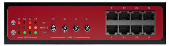
Figure 14: LEDs E1 – E4
