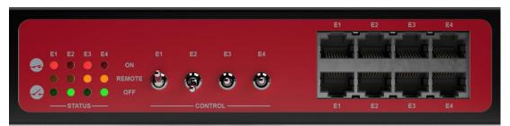
Figure 3: Ethernet relays E1 - E4
